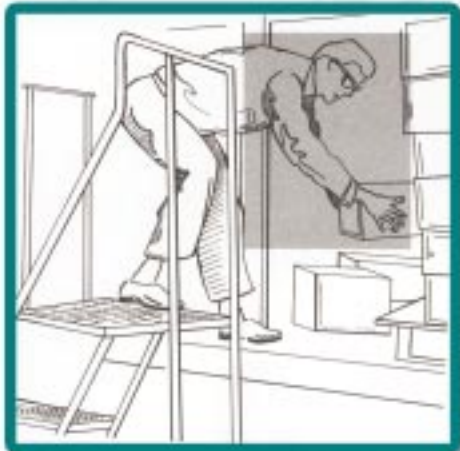
Do not lean off ladder.
