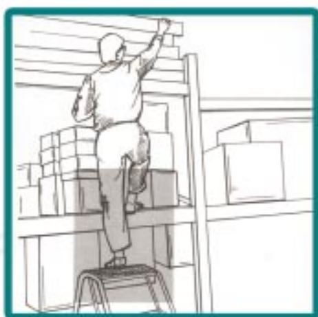
Do not climb off the ladder.
